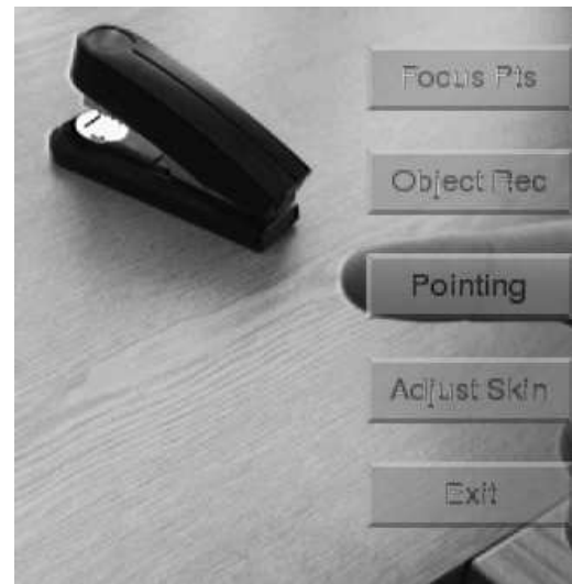
Figure 4: Menu control by fingertip: The user carries out a “pressing” gesture on a button. The system analyzes the position and the movement trajectory to recognize “Selected” and “Pressed” events.
