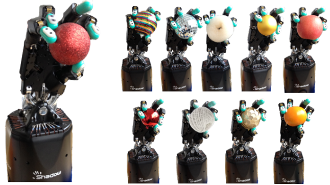
Fig. 1. This figure shows the uniform in-hand objects considered as Prior Objects. The Shadow Hand with the BioTac sensors is exploring the texture properties of the in-hand objects with an identical shape. It moves any of the fingertips to slide over the objects surface and uses the proposed tactile descriptors to extract robust tactile information.
