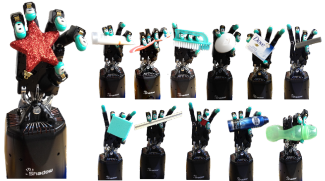
Fig. 2. This figure demonstrates the complex shape in-hand objects considered as New Objects. Employing the proposed tactile transfer learning the Shadow Hand discriminates new objects from their texture with a very few trials whilst re-using prior knowledge.
