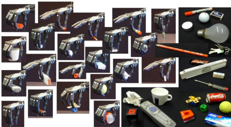
Figure 2: Example grasps (left) of the Shadow Hand with the algorithm from [59] for a benchmark collection of 21 common household objects (shown on the right).
